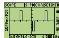
While the horizontal sweep of the scope doesn't go lower than 10 Hz, the scope's response goes down to DC, so it will show the presence (and effect of) a DC offset. A pause button allows you to freeze the scope display for closer examination.
