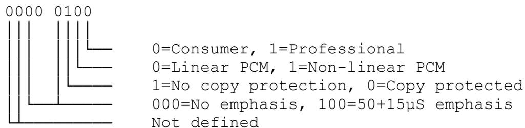
In the Consumer format, the sample rate is defined in the four lowest order bits of byte 3 (0000 = 44.1 kHz), and other bits define the generation of the recording, which in turn defines whether a digital copy can be made.
