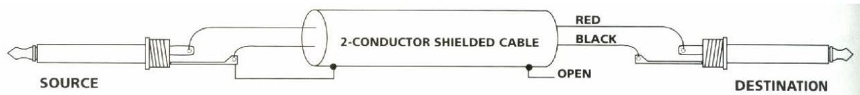
Fig. 2 - Wiring Unbalanced Connectors (One-end-only grounding)
