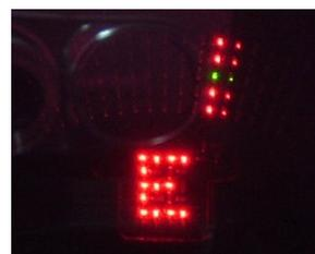
When a string is much further off pitch than a half-step, the green LED in the “on pitch” arc will either blink or disappear.
