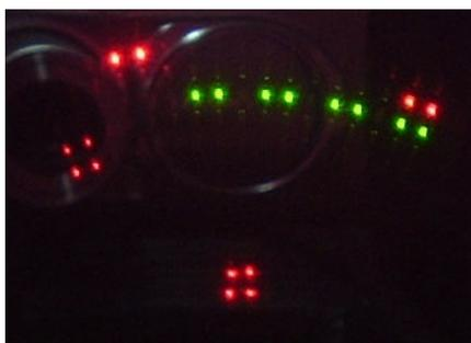
Here's the polyphonic display with a mono display of each of the three out-of-tune strings below. As you can see from the LED matrix, the poly display has two steps above and below the correct pitch. Note that the A string, being pretty sharp, is at the second "off pitch" step. This is sharp enough to be interpreted as being A# and a little flat
