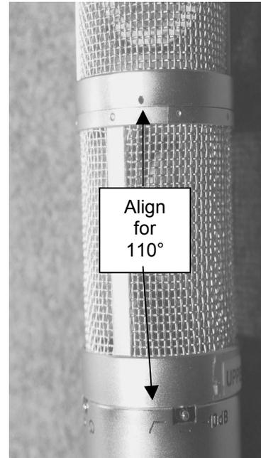
With the upper capsule rotated to this position, the center line for the pair is located at 55 degrees. Again, there's no dot to mark this, but it's in line with the cardioid marker for the lower microphone switch. Aim that
