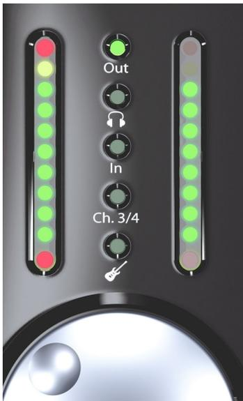
The operating concept is simple. If you want to adjust the monitor volume, click the knob until the **Out** LED is illuminated. Turning the knob then controls the level for Outputs 1-2. Similarly, if you want to adjust the gain of the mic inputs, click the knob until the **In** LED illuminates and the knob becomes the Input 1-2 gain control. To adjust the headphone volume, click down to the **phones** LED and turn the knob, or .
