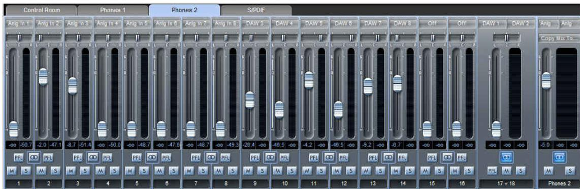
This screen shot shows a headphone mix consisting of the analog inputs 1-8 plus six mono DAW outputs. The "main" DAW outputs (DAW 1 and DAW 2) also appear in this mix since we want to use them in the Control Room mix, but in the
