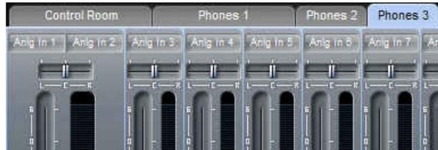
stereo mixes here, but we could have eight mono mixes, each with its own tab, or we could have some stereo (Control Room and Phones 1) and some mono mixes (Phones 2 and Phones 3) as shown above. The limitation is that there are only eight physical outputs so that's the maximum possible
