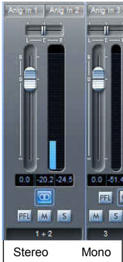
Consecutive input pairs can be configured as a stereo channel with a single fader to adjust the level of both channels simultaneously.
