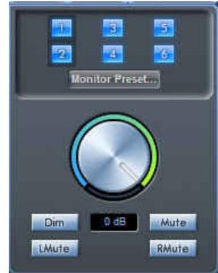
Clicking on one or more of the numbered buttons turns it red and mutes that output. Shift-clicking a numbered button (they turn sort of gray) disables the Mix Control volume knob and sends the full signal level to all of the hardware volume controls. For studio use with the 18i8 within reach, I found this to be the most useful setting. The front panel knobs work as expected, and you won't wonder where your monitors went if you inadvertently change the software monitor control knob.
