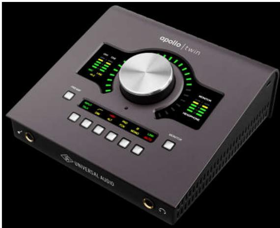
Universal Audio released the Apollo Twin MkII, a significant makeover of this popular and powerful desktop Thunderbolt-connected interface. Significant updates include new technology A/D and D/A converters for lower distortion and increased dynamic range, and incorporation of their Unison mic preamp modeling technology, which adds emulation of several classic mic preamps to the Apollo's mic and instrument DI inputs. In addition to the two front panel
