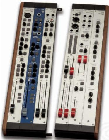
you to custom-assemble your own console. They offer two line/mic input modules, one standard and the other "ultra low noise," a high input impedance instrument DI input module, a stereo line level input module, and two master modules. The frame is sectional, so you can assemble whatever size you need.
