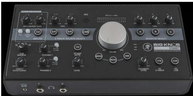
At this show, Mackie re-introduced the Big Knob monitor controller, in three versions this time around. The Passive is a true passive pot in a box offering a selection of two stereo input sources and two stereo outputs, mute and dim switches, and a big volume control knob. The Studio
