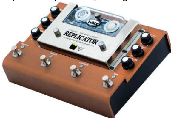
There’s an erase head, a single record head, and two playback heads that can be switched to either provide two different delay times, or one can be switched to feed back to the record path to create repeating echoes. Delay is adjusted by varying the tape speed, which suggests that long delays might suffer a little loss of high frequency
