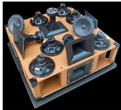
The top cabinet has four horns, one on each side, with ports on each corner. Each horn is powered by its own 250 watt amplifier. This is paired with a bass rotary cabinet with eight 8" drivers with 250 watts powering each pair. The photo shows the complement of speakers in the top and bottom cabinets. For extra bass power, there's a non-rotary sub-bass
