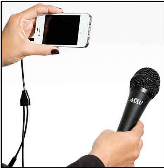
This is a cable-connected mic with a splitter for connecting headphones.
