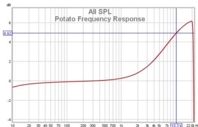
Here's a plot of the frequency response of a representative potato. It's quite flat up to 1 kHz, where it begins rising to about +5 dB at 20 kHz. Since there isn't much above about 5 kHz coming out of a guitar amplifier, the high frequency rise is probably negligible. Sylvia also mentioned a rising high frequency response, so it's good to know that at least someone else observed what I measured what and found similar results.
