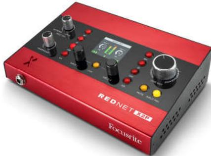
The Focusrite RedNet X2P is a desktop form factor 2-in by 2-out audio interface with two Red Evolution mic preamps. Mic/Line inputs are on XLR-TRS combo jacks, main analog output with a hefty +24 dBu maximum output level is on XLRs, and a front panel 1/4" TRS jack with an independent volume control provides a headphone output. Computer connection is via Dante, with power supplied either through the Ethernet cable from a PoE (Power over
