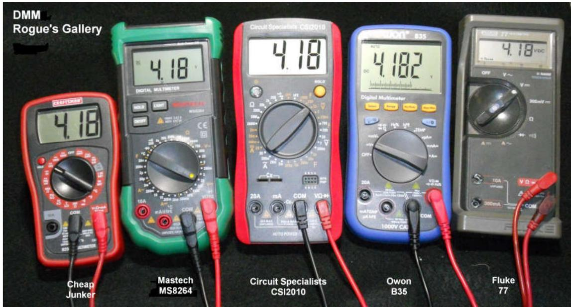
For this photo, all of the meters are connected to the same power supply and, as they should, all read the same to the extent of their resolution. Note that the Owon has one more digit after the decimal point than the others. This is because it has a larger “half digit” than the rest.
