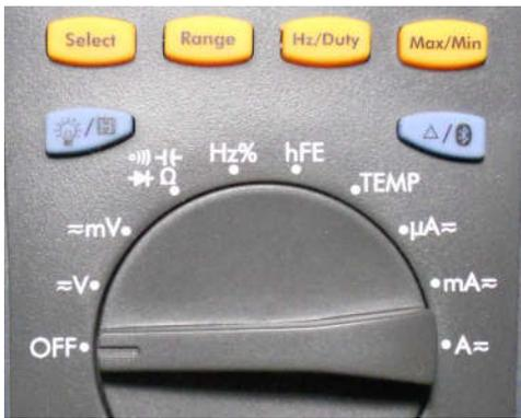
The two manual-ranging meters have a pretty straightforward user interface, but the auto-ranging Owon is rather different. With manual range switching, you switch to what you want to measure, then, other than perhaps moving a test lead to a different jack for measuring a capacitor or high current, you're good to go. The Owon (pictured at left) puts me slightly in mind of a digital mixing console or DAW software program - making just about any setting requires using two controls.
