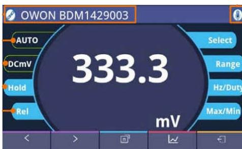
The Owon has the unique feature of a Bluetooth remote display and remote control. This deserves a review of its own so I'll be brief here. Pairing the meter with a dedicated Android or iOS app allows you to read and operate the meter remotely. In addition to providing a remote display, it can use your mobile device's text-to-speech to read the displayed value to you, log readings at
