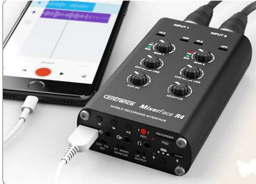
inputs and DAW playback when overdubbing. The mic inputs have 48v phantom power available and there's a switchable low-cut filter. The rig is powered by an internal rechargeable battery which they claim gives 8 hours of service on a charge. Computer interface is USB, class compliant with iOS and (some) Android phones, it can record to a Micro-SD memory card.
