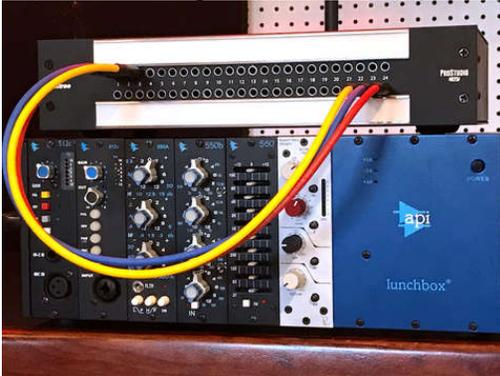
Radial 6-Pack. It offers two rows of 24 bantam jacks which can be set with jumpers hidden behind the label strips for full normal, half normal, or no normal connections between the top and bottom rows. Connections on the rear panel are with TASCAM-wired DB-25 connectors in groups of eight. At \$625, it's not cheap, but that's about half the price of one of their full rack sized panels.
