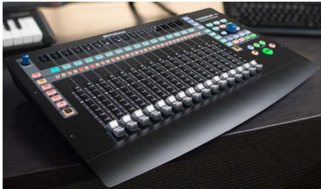
The motorized touch-sensitive 100 mm long faders feel good under the fingers and move quietly. Like the other FaderPorts, it's pre-programmed for either HUI or Mackie Control, one or both of which practically all of this generation's DAWs understand. Naturally, it has some special features that integrate tightly with PreSonus' Studio One DAW software, though it's been tested with several DAWs – Pro Tools 12, Sonar, Logic 10.4, Cubase 9.4, Harrison Mixbus, and others.
