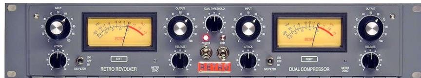
two-channel compressor, the Revolver. It's based on an Altec 436B single channel variable mu broadcast compressor, incorporating modifications by engineers at EMI Abbey Road Studio in the 1960s. The name comes from the fact that these compressors saw a lot of use in recordings of The Beatles. Beatles-Revolution-Revolver – get it?
