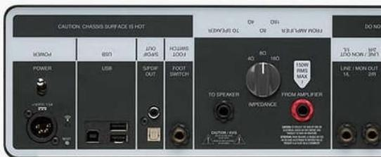
All of the gozintas and gozoutas are on the rear panel. Cleverly, they've printed the labels both in the normal orientation and upside down, so you can read them when looking down on it from its intended position on top of the amplifier.
