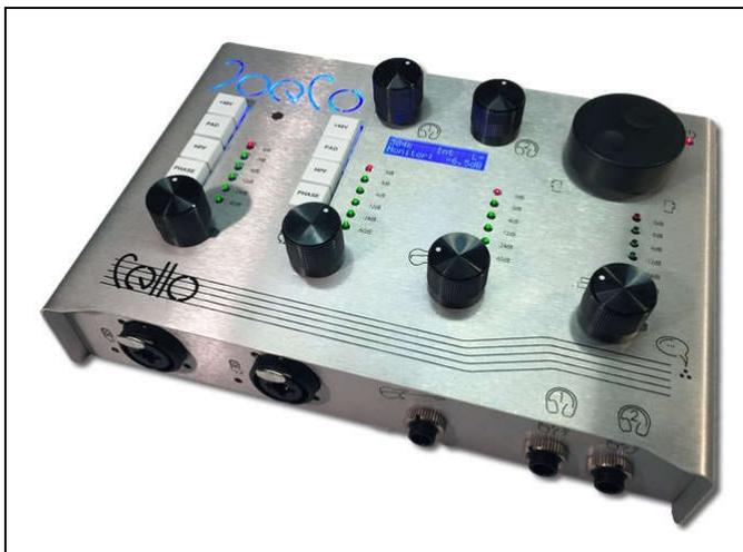
There are two mic-only input channels with low cut filter, polarity reverse, pad, 48v phantom power, and line level inserts for outboard analog processing. There are also two ADAT optical inputs, S/PDIF input, an instrument DI with its own 1/4" jack and level control, and four outputs. For studio applications, there's a built-in talkback mic and a monitor mixer. There's little technical data available at the moment,
