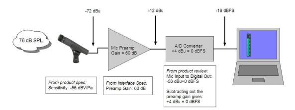
If we're aiming for 16 dB of headroom, the DAW meter shows that we're occasionally using most of that. In this case, it took all of the preamp's gain to reach a decent record level. Replace the soft voiced narrator with a powerful rock singer and the preamp gain will need to come down by 20 dB or more in order to avoid overloading. Replace the SM57 with a hot condenser mic, and you might have to switch in a 20 dB pad. And that, folks, is how it works in the real world.
